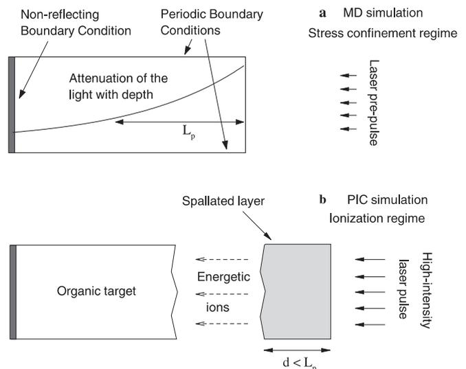
**Fig. 1a,b.** Schematic sketch of the simulation setup
