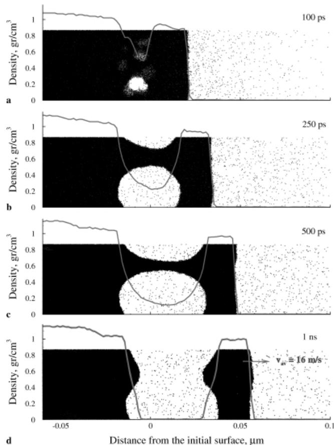
**Fig. 2a–d.** Density profiles near the surface of irradiated sample for simulation with 15-ps laser pulse and fluence of  $31 \text{ J/m}^2$ . Corresponding snapshots from the simulation are shown in the background of the density plots
