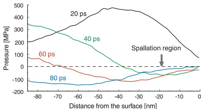
**Fig. 3.** The spatial distribution of pressure in the MD computational cell at different times following irradiation by 15-ps laser pulse at laser fluence of  $31 \text{ J/m}^2$ . Snapshots from the simulation are shown in Fig. 2. Non-reflecting boundary condition is applied at the depth of  $-90 \text{ nm}$  as shown in Fig. 1
