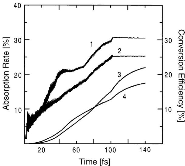
**Fig. 5.** Temporal evolution of the absorption rate, (1) and (2), and the conversion efficiency of the energy of the laser pulse to the energy of ions, (3) and (4), for a 25-nm spalled layer, separated by  $1 \mu\text{m}$  from the target and irradiated with 100-fs laser pulse at wavelength of 400 nm and intensity of  $10^{17} \text{ W/cm}^2$ , (1) and (3) and  $10^{18} \text{ W/cm}^2$ , (2) and (4)
