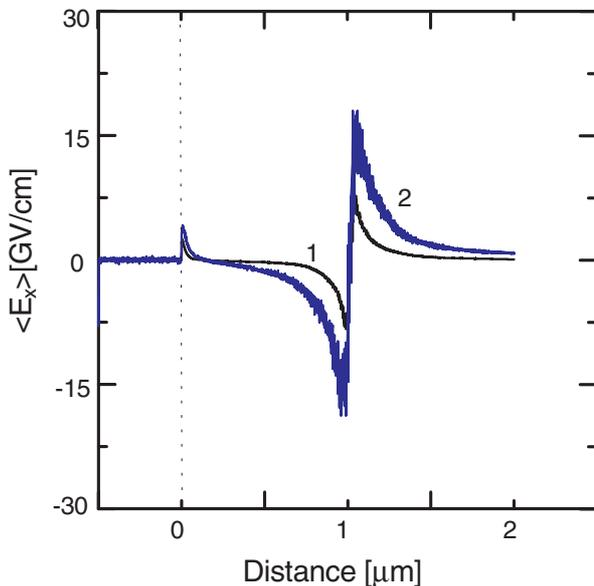
**Fig. 7.** Spatial distribution of the temporary averaged electric field, (1)  $I = 10^{17}$  W/cm<sup>2</sup> and (2)  $I = 10^{18}$  W/cm<sup>2</sup>
