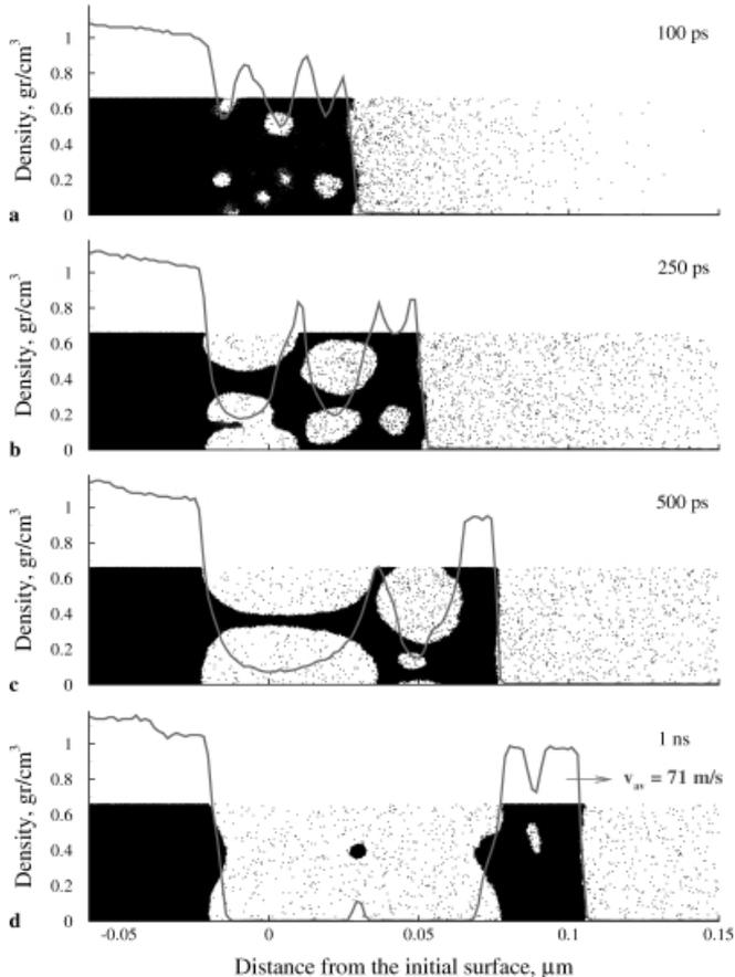
**Fig. 4a–d.** Density profiles near the surface of irradiated sample for simulation with 15-ps laser pulse and fluence of  $34 \text{ J/m}^2$ . Corresponding snapshots from the simulation are shown in the background of the density plots
