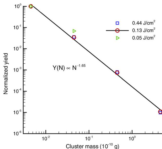
Fig. 2. Normalized mass distribution of particles deposited in MAPLE at fluences of 0.05, 0.13 and 0.44 J/cm<sup>2</sup>. The threshold fluence for deposition of polymer particles is 0.045 J/cm<sup>2</sup>. MAPLE target is 5 wt.% PMMA solution in toluene. A power-law dependence,  $Y(N) \propto N^{-1.65}$ , where  $N$  represents the mass of the deposited particle, describes well the results for large surface features obtained at all three laser fluences.
