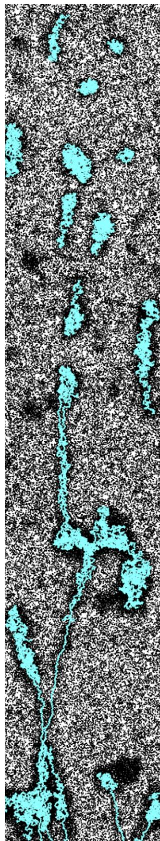
Fig. 3. Snapshot from a MD simulation of MAPLE with a target containing  $6 \text{ wt.}\%$  of polymer. Laser fluence is  $9 \text{ mJ/cm}^2$ ,  $\sim 60\%$  above the ablation threshold. Matrix molecules and units of polymer chains are shown by black and blue dots, respectively. The polymer chains are superimposed on top of the image of matrix molecules shown in the background.
