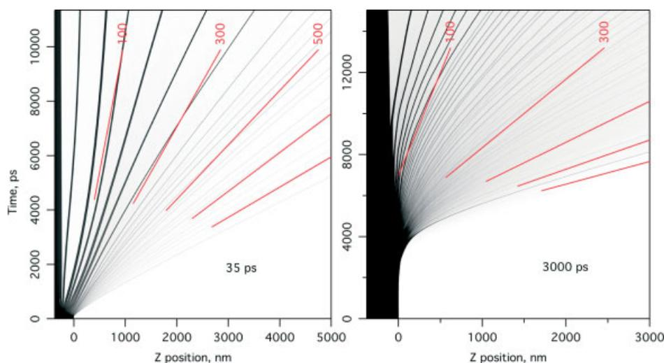
**Figure 3.** Laterally projected density versus time for samples irradiated with  $50 \text{ mJ/cm}^2$ , 355-nm laser pulses, of two different  $1/e$  full widths: 35 ps, and 3 ns. The density scale is as in Fig. 2. Lines representing velocities of 100, 300, 500, 700 and 900 m/s are plotted radiating from a single point or depth, for comparison to the trajectories of the ejected material.
