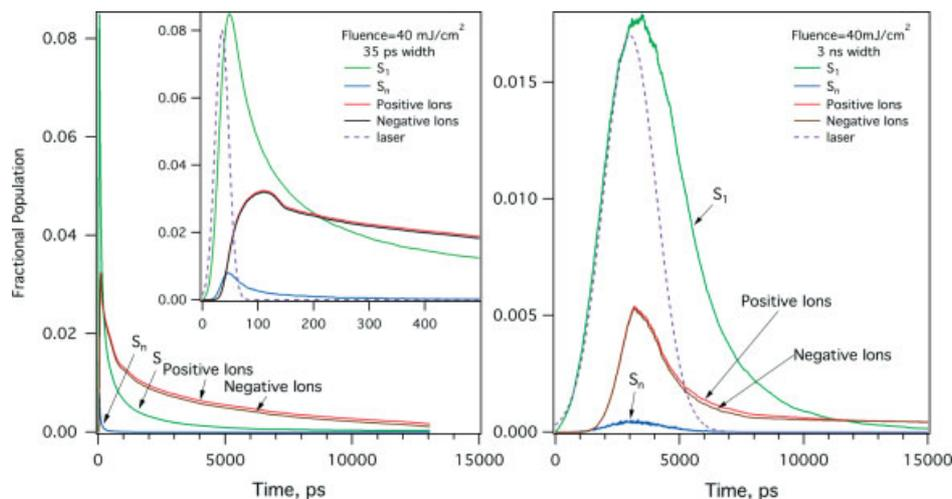
**Figure 1.** Evolution of matrix excited states and ions versus time, for 355-nm laser pulses of two different full widths: 35 ps and 3 ns, at a fluence of  $40 \text{ mJ/cm}^2$ . Ion formation and ablation are largely sequential for short pulse excitation, whereas they overlap considerably for the longer pulse length.
