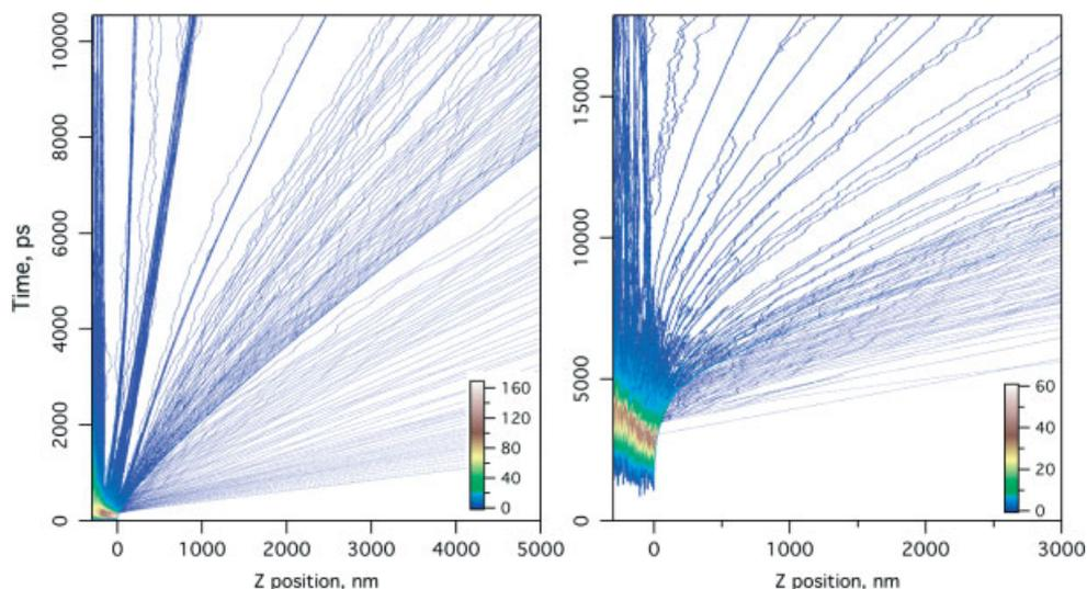
**Figure 9.** Laterally averaged charge density versus axial position and time, for the two simulations of Fig. 8. All charges are summed, positive and negative charges do not cancel. Note that the color scale spans different ranges for the two panels.
