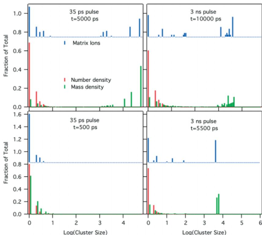
**Figure 10.** Normalized cluster size, mass and matrix ion histograms for short (35 ps) and long (3 ns) laser pulses, at early and late times. The fluence was  $40 \text{ mJ/cm}^2$  in both cases. The ion histograms represent the masses of clusters in which one or more matrix ions are found. The mass-weighted histograms have been slightly laterally shifted for clarity.
