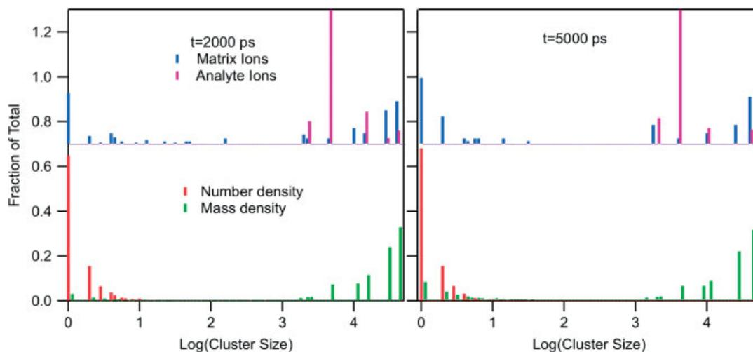
**Figure 12.** Histograms for the simulation of Fig. 11. Both matrix and analyte cluster ion histograms are shown, representing the sizes of the clusters in which ions are embedded. The mass-weighted and analyte ion histograms have been slightly laterally shifted for clarity.
