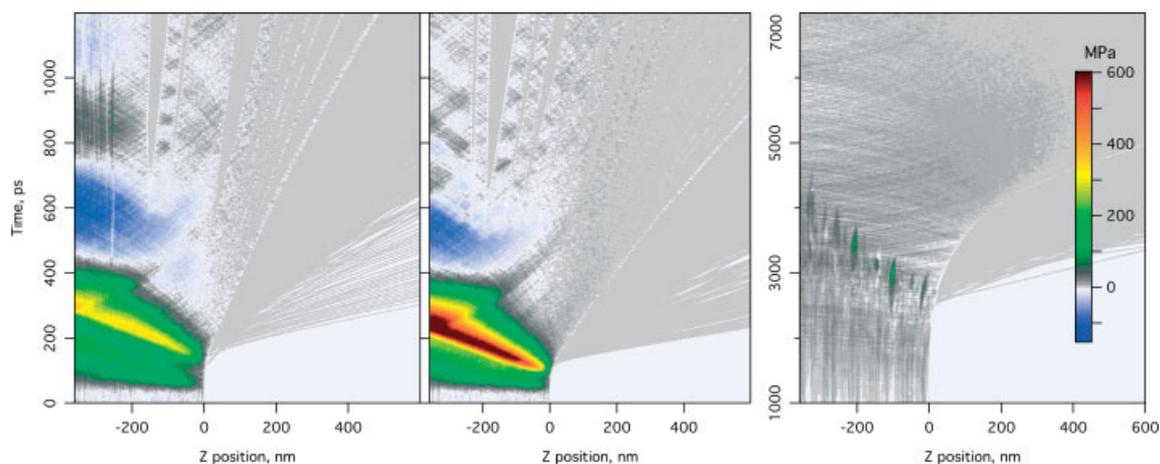
**Figure 4.** Laterally averaged pressure versus time, in Pascal. The left two panels show results for 35-ps laser pulse widths, of 40 (left) and 50 (middle)  $\text{mJ}/\text{cm}^2$ . The right panel shows results for a 3-ns, 50  $\text{mJ}/\text{cm}^2$  laser pulse. The color-coded pressure scale is the same for all panels.
