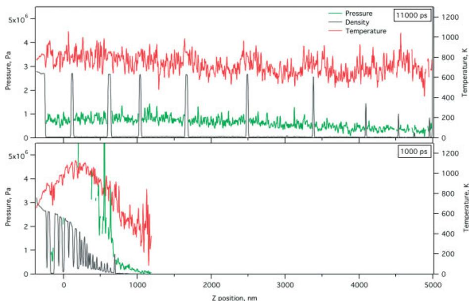
**Figure 5.** Snapshots of pressure, temperature and density versus axial distance for a 35 ps, 50 mJ/cm<sup>2</sup> laser pulse, at early and late times in the simulation. The pressure traces have been masked to show only the gaseous regions. The temperatures are calculated using only the lateral velocities, so as not to be distorted by the axial stream velocity. Regions of very low density, with too few molecules for a meaningful average, are also blanked.
