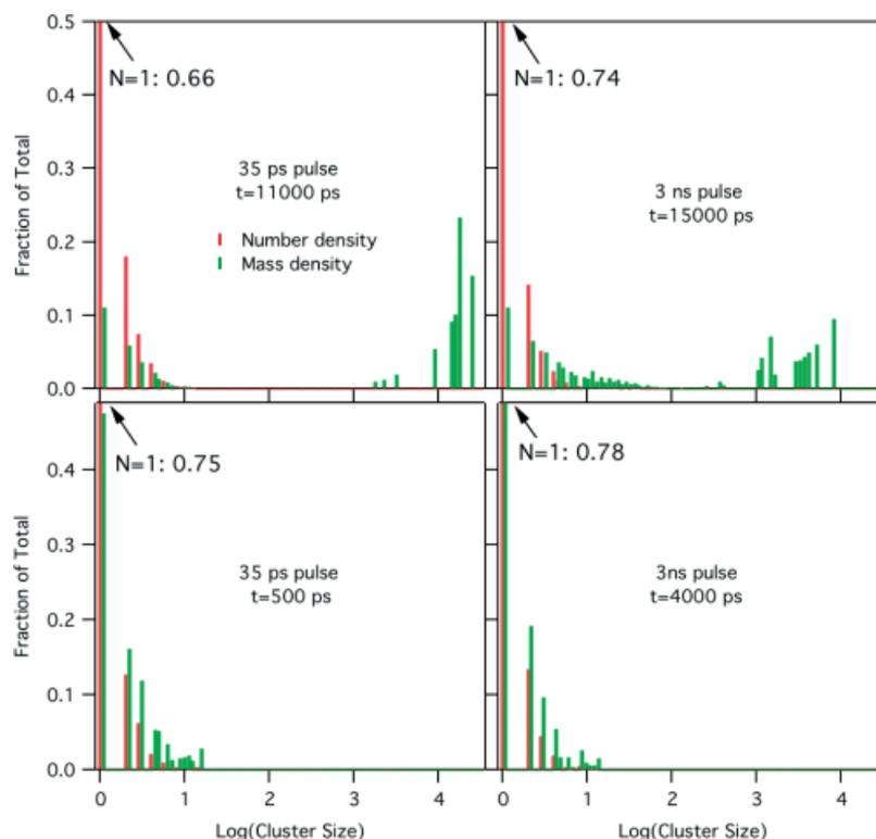
**Figure 8.** Normalized cluster number and mass-weighted histograms for short (35 ps) and long (3 ns) laser pulses, and early and late times. The fluence was  $40 \text{ mJ/cm}^2$  in both cases. The mass-weighted histograms have been slightly laterally shifted for clarity.
