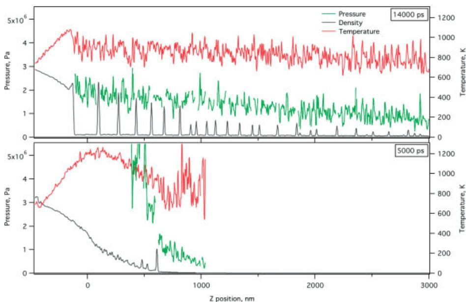
**Figure 6.** Snapshots of pressure, temperature and density versus axial distance for a 3-ns laser pulse, at 50 mJ/cm<sup>2</sup>. The pressure traces have been masked to show only the gaseous (low density) regions. The temperatures are calculated using only the lateral velocities, so as not to be distorted by the axial stream velocity. Regions of very low density, with too few molecules for a meaningful average, are also blanked.
