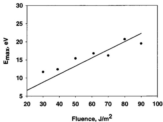
**Figure 5.** Maximum value of the internal energy of that analyte molecule embedded at the depth  $Z_0 = -42 \text{ \AA}$  as a function of laser fluence. Calculation results are obtained at  $t = \tau = 150 \text{ ps}$ . The line is a linear fit to the dependency.
