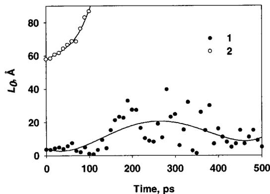
**Figure 6.** Distance between the end beads of the analyte molecule (the length,  $l_0$ ) as a function of time. Calculations are performed for laser pulse duration  $\tau = 300 \text{ ps}$  and laser fluence  $F = 90 \text{ J/m}^2$ . (1) the molecule is initially unextended; (2) the analyte molecule is initially extended in the direction perpendicular to the irradiated surface. At  $t = 110 \text{ ps}$  the first molecule is broken. Lines are just guides to the eye.
