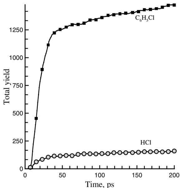
Fig. 2. Plot of the total yield of molecules as a function of time. Other species namely  $C_{12}H_8Cl_2$ ,  $C_6H_6$ ,  $C_6H_4Cl_2$  and  $Cl$  are not presented in the plot because of the small concentration (less than 10 molecules).
