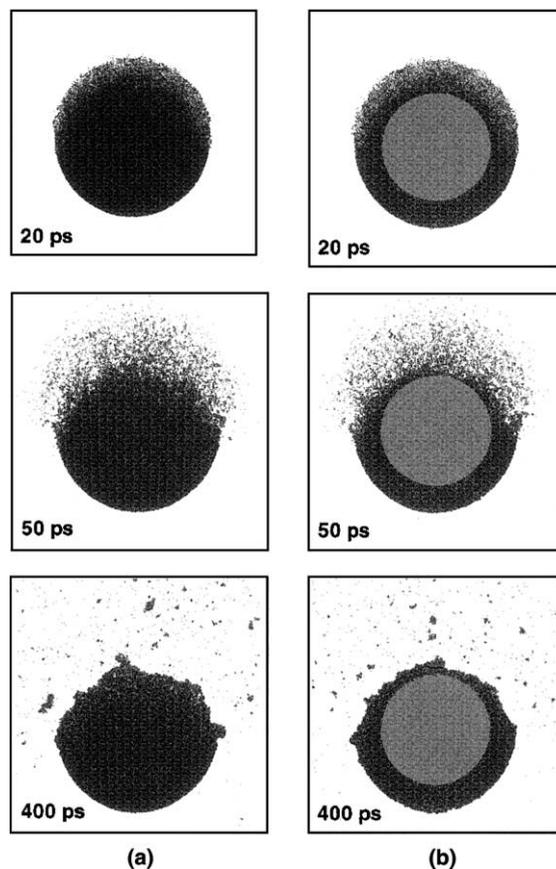
Fig. 1. Snapshots (20, 50 and 400 ps) of the amorphous particles subjected to a laser fluence of 25 eV/nm<sup>2</sup>. The laser irradiation is coming from the top of the page. (a) Particle without inclusion. (b) Particle with transparent inclusion where the diameter of the particle is 1.5 times the diameter of the inclusion.
