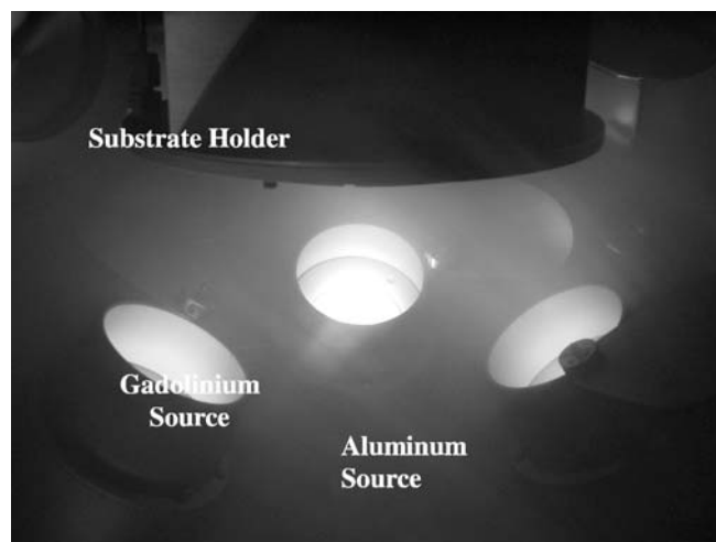
FIGURE 1 Digital photograph of the 3-source configuration for the combinatorial sputter deposition process
