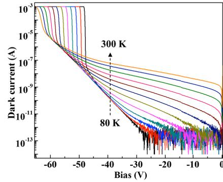
Fig. 5. Current-voltage curves of a  $50 \mu\text{m}$  device for temperature 80 K to 300 K in 20 K steps.
