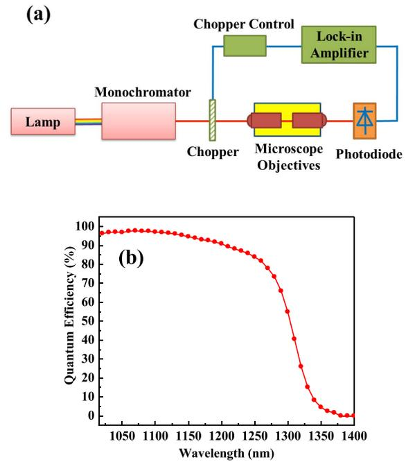
Fig. 3. (a) Quantum efficiency measurement setup; (b) measured quantum efficiency of a device with diameter of 250  $\mu\text{m}$ . The bias voltage is  $-5 \text{ V}$ .
