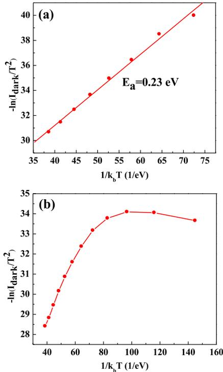
Fig. 6.  $-\ln(I_{\text{dark}}/T^2)$  versus  $1/k_b T$  for a  $50 \mu\text{m}$ -diameter device at (a)  $-10 \text{ V}$  and (b)  $-35 \text{ V}$ .
