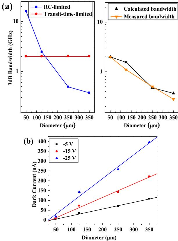
Fig. 4. (a) Calculated and measured bandwidth versus diameter at bias voltage of  $-5$  V; (b) dark current versus diameter at different bias voltage.
