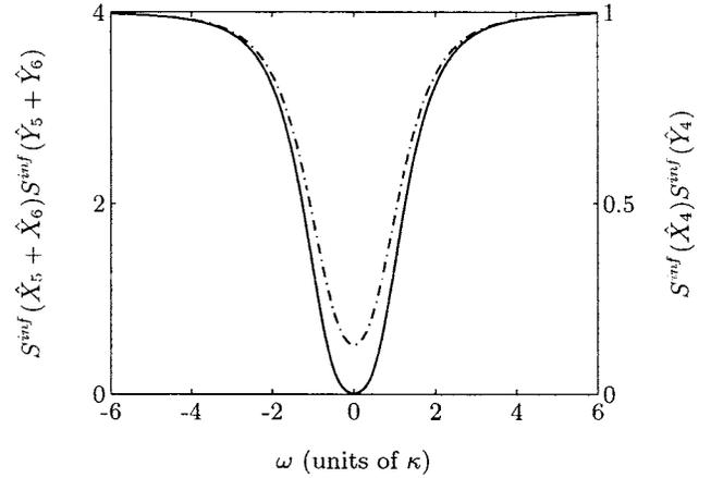
FIG. 4. Output fluctuation spectra of the inferred quadratures for three-mode EPR correlations, from measurements on one or two modes. Below threshold ( $E=0.9E^{\text{th}}$ , solid line) the spectra coincide. Above threshold ( $E=1.1E^{\text{th}}$ , dash-dotted line) two-mode inference gives better violation than one-mode inference, but the difference is indistinguishable on this scale.
