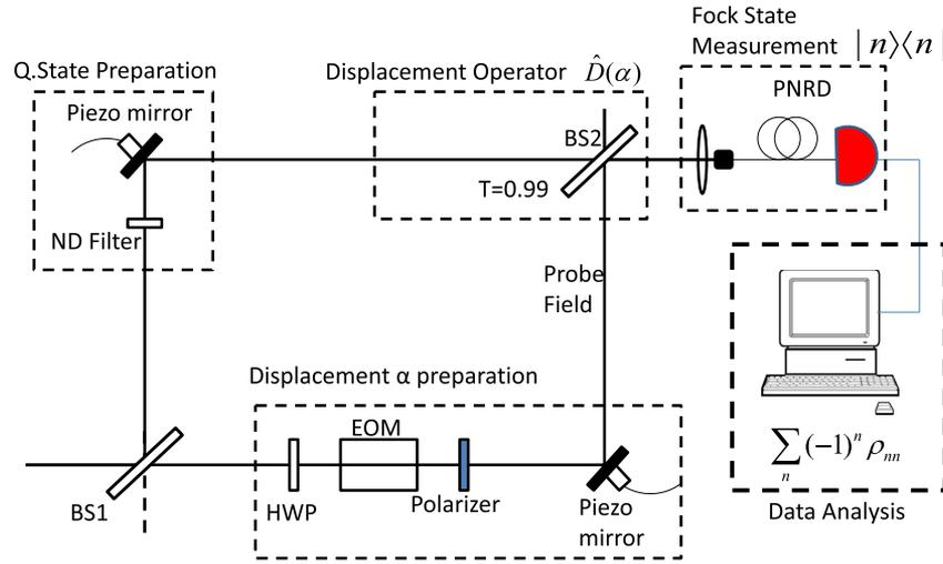
Fig. 6. Experimental setup for the quantum tomography of a coherent state using a coherent probe field and photon number measurements. The leftmost and upper optical path is that of the quantum state to be measured. The lower and rightmost optical path is that of the “local oscillator” whose field generates the phase-space displacement. BS, beam splitter; EOM, electro-optic modulator; HWP, halfwave plate; ND, neutral density.
