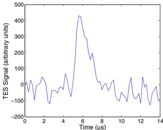
Fig. 2. Example of raw TES data showing a single photon detection event. The detection peak can be clearly distinguished from the noise.
