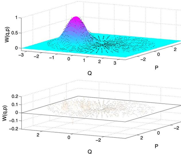
Fig. 8. Gaussian fit (top) and residuals (bottom) of the coherent-state tomographic data. The fit function was  $W_{\text{fit}}(q, p) = a + b \exp[-m|(q - q_0)^2 + (p - p_0)^2|]$ . The correlation coefficient was  $R^2 = 0.966$ .
