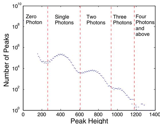
Fig. 5. Histogram of peak heights from the sample of Fig. 4(a). The histogram bins define the photon-number quantization thresholds.
