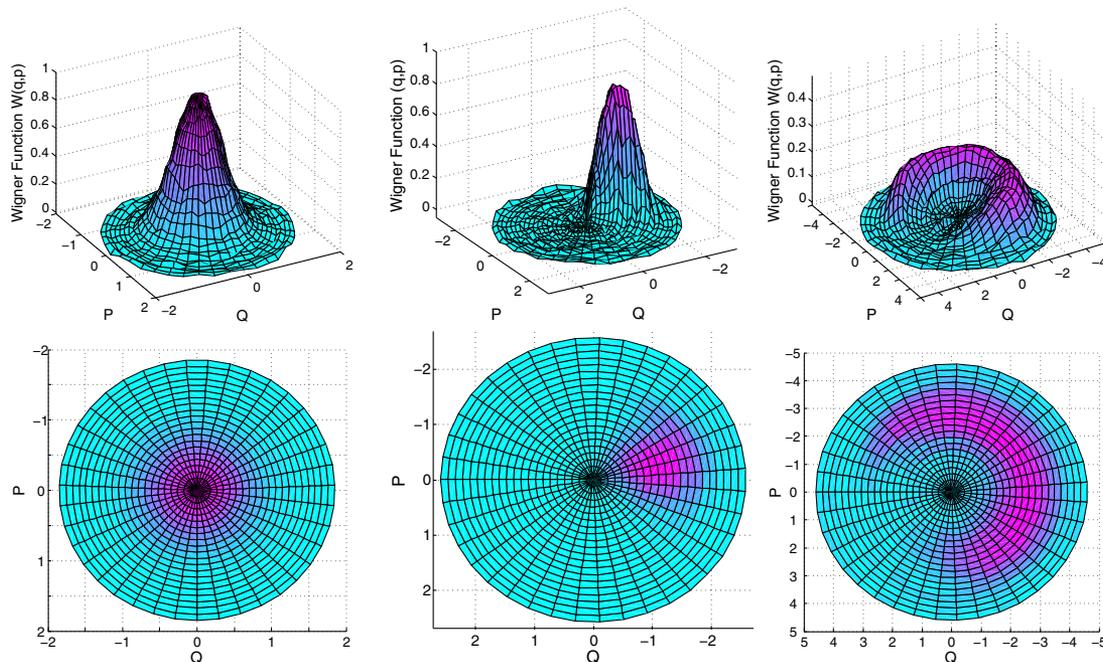
Fig. 7. Measured Wigner functions and contours of vacuum (left), coherent state (center), and phase-diffused coherent state (right). All plots are interpolated for 22 amplitude points and 40 phase points.
