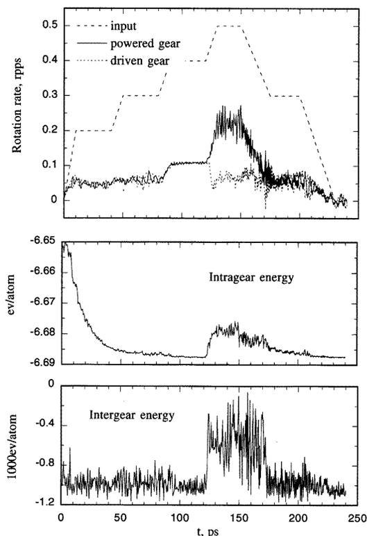
**Figure 3.** Rotation rate and energy for gear simulation with temperature control.
