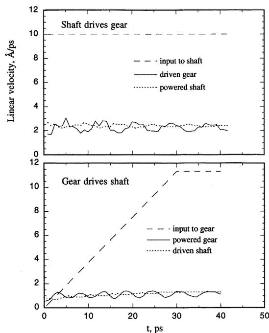
**Figure 8.** Velocity of gear and shaft configuration.
